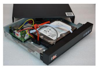
Secure the hard disk with the 4 screws provided. they screw from under the VCR
