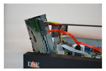
Connect the hard disk with the two cables power and data that you find inside. If there there are multiple doors, choose any pair.
